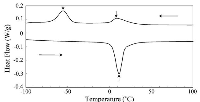
**Fig. 3** DSC curve of as-received wire
