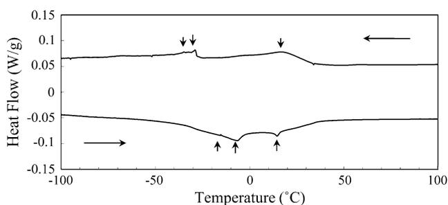
**Fig. 7** DSC curve of solution treated and aged wire at 400 °C for 30 min
