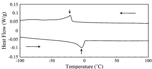
**Fig. 5** DSC curve of solution-treated wire
