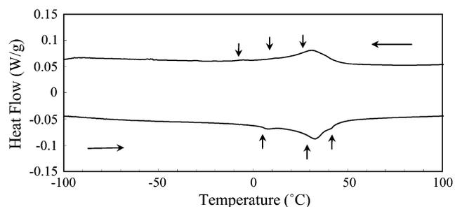
**Fig. 8** DSC curve of solution treated and aged wire at 400 °C for 60 min
